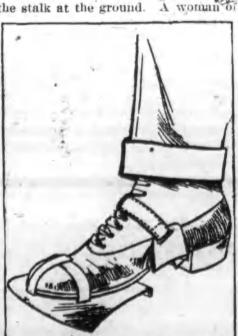
Navasota, Tex., has remedied this in a device to be secured to the farmer's shoe by which the cutting is done with a quick movement of the foot and no leaning over is required. The knife is a broad, flat blade secured to the shoe at the toe and over the instep and braced for the repeated blows it will receive by ending against the heel.
