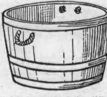
saw the barrel through the middle in order to have a receptucle which will hold one bushel.
